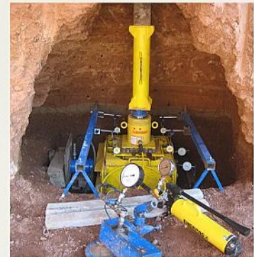
▲ In situ direct shear test, Tarlan complex
